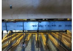
7. The beater hits the woven fabric as it wraps around the front beam on it's way to the front cloth beam when the warp is advanced more than an inch or two. This makes the possible weaving area very narrow which slows weaving and demands multiple advances. If this is not watched VERY CAREFULLY, the beater hits the woven weft and leaves large gaps in the woven weft.
